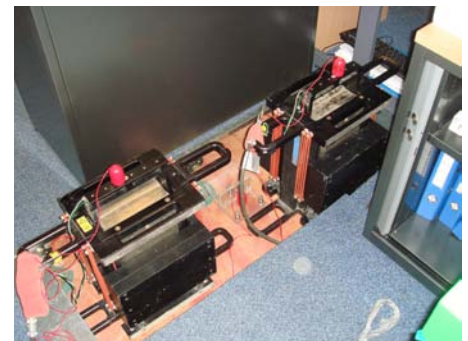
Figure 11 Active vibration control system in operation: (left) simulating excitation with one shaker while controlling with another.
