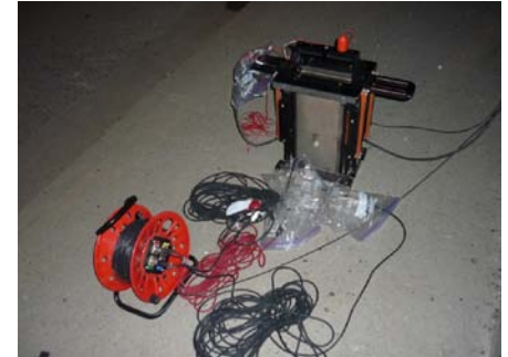
Figure 1: Shaker and accelerometers on bridge during forced vibration test.
